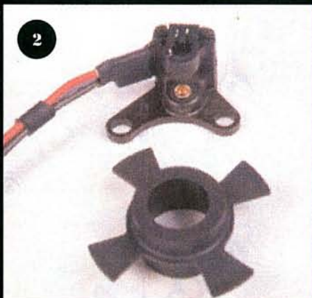
4 If you don't want to drill any holes in the bodywork, Lumenition also supply this neat bracket that mounts the module next to the coil using the coil's original mounting holes.
